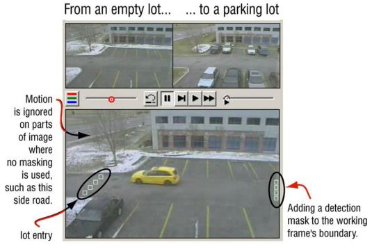
**Fig. 53.** Masking the entrance/exit to a parking lot. You can search for arrival and departure times by using masks at entry points to an area, and/or at the boundaries of an image. Use of a mask excludes unmasked areas from being searched for movement.
